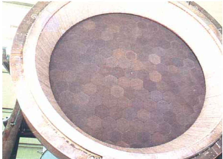
Figure 8 Volumetric receiver (Source: DLR)
