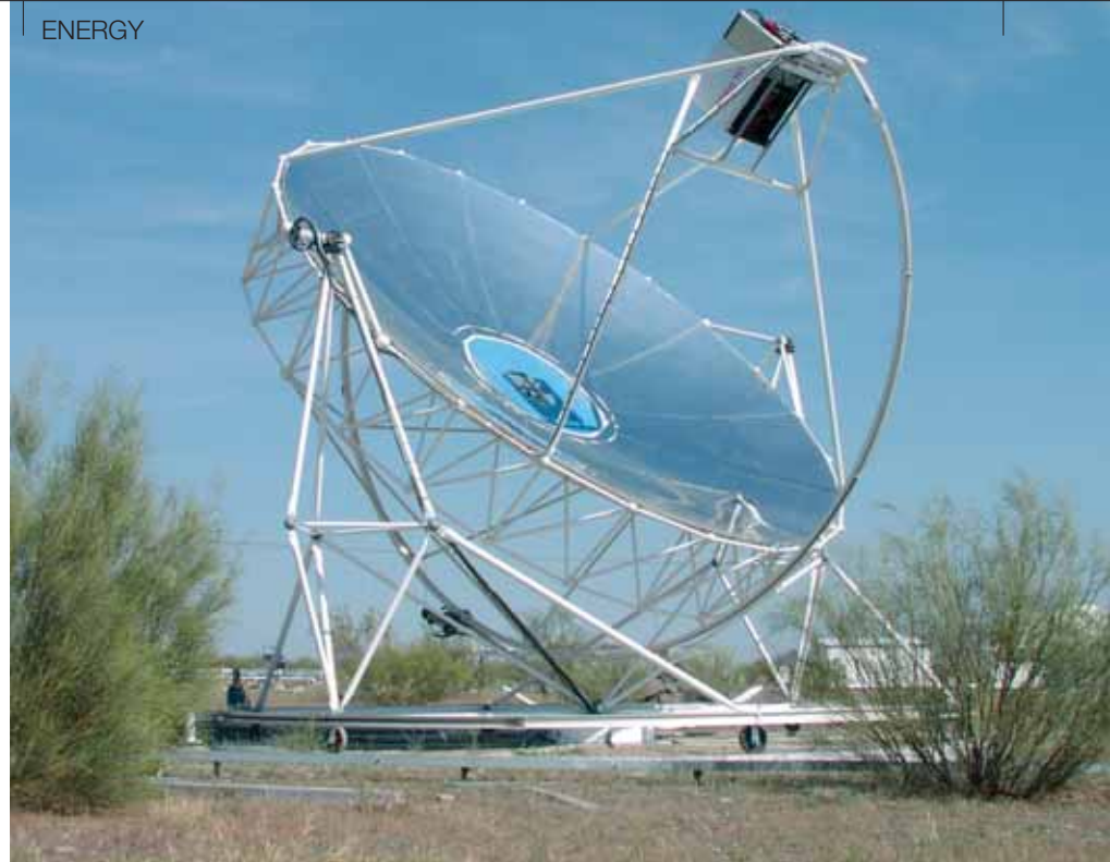
Figure 6 The EURO-DISH parabolic dish concentrator with a Stirling motor-generator in the focal point at the CIEMAT solarthermal test centre Plataforma Solar de Almería, Spain (Source: SBP)
