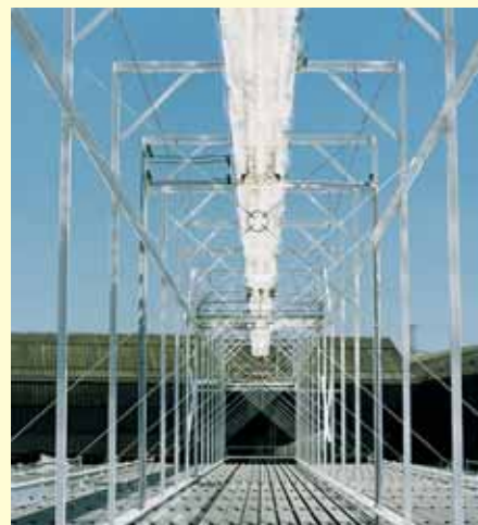
Linear Fresnel collector at the Solarmundo test facility in Liege, Belgium
